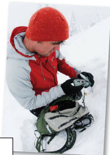
Taking slope angle measurement.
